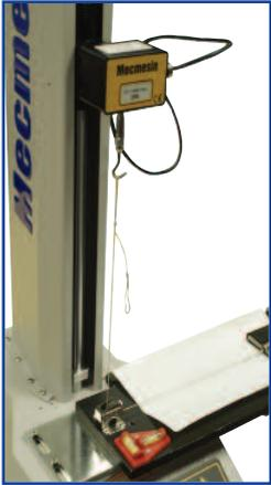
1. A horizontal test table is fixed to the stand, with one test specimen attached to the test table and another laid directly on top. A sled of known mass is positioned in the centre of the test specimen and attached to the crosshead of the stand.
