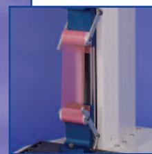
Mecmesin also offers the option to use your COF tester as a tensile testing system, which is ideal for measuring the strength of materials such as plastic film. Forces applied during the production process can be replicated to assess stretch resistance and durability of materials.
