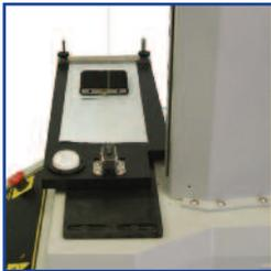
3. The force required to begin movement of the sled (static force), and the force used to keep the sled in motion (kinetic or dynamic force) are displayed and coefficients are automatically calculated at the end of the test. Using Emperor software, results can then be exported to a printer or a PC for further analysis.
